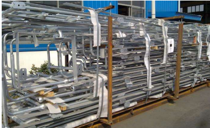
Figure 15: Light steels such as handrail – non-stackables
